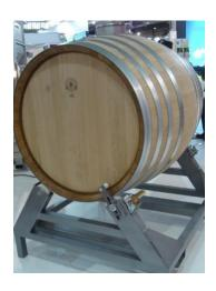
The rotative micro fermenter enables a gentle stirring thanks to the rotation (without crushing grapes skins and seeds).
